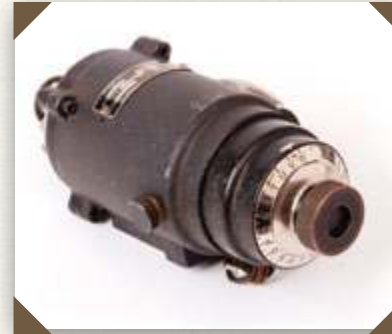
Adjustable-speed motor with a governor
